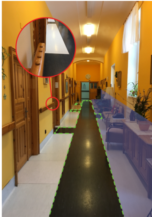
Figure 2.10: A corridor in Palata. Red zoom shows the haptic marks, dashed green line contrast the navigation line, blue color marks the furniture for the resting, from [32]
